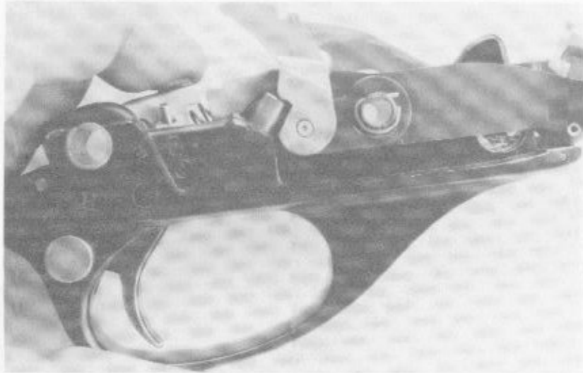
Right side view showing a close-up of the newly converted trigger mechanism. Selector is set on "semiauto." Photo shows the automatic tripper being depressed but not pulling the trigger. To prevent accidental discharge, make sure that the hammer is not tripped which may be caused by heavy rubbing of the automatic tripper and the trigger when assembled together in the frame.
