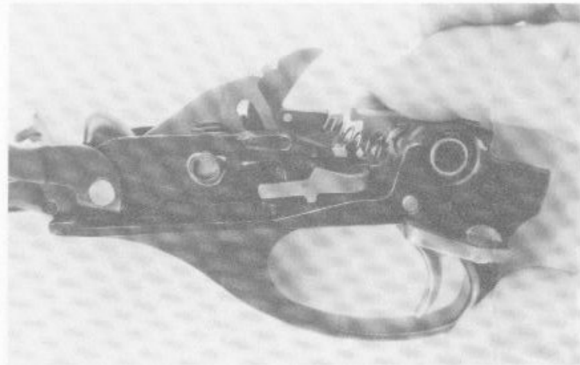
Another view showing the tripper being depressed without tripping the hammer sear. The trigger is not pressed and the selector is set on "full auto." This is the relationship of parts during the loading process without the trigger being pulled and with the selector being set on any index. For maximum safety, the shooter must make it a habit to set the selector on "safe" each time he loads the weapon or when he is not ready to fire.
