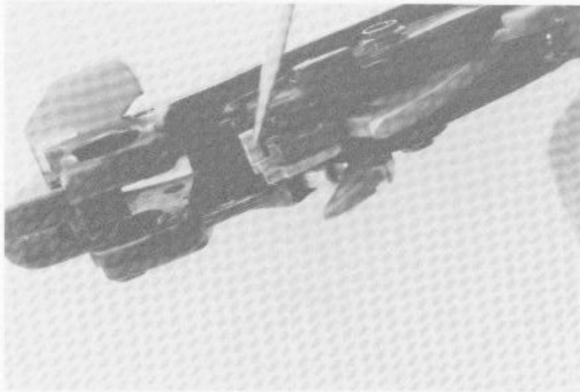
Scribe points to the lower bent part of the sear extension. This portion of the extension rides over the center step of the modified sear. When the sear extension step is depressed by the tripper, this bent part of the extension will depress the sear causing the hammer to be released, thus firing the weapon.
